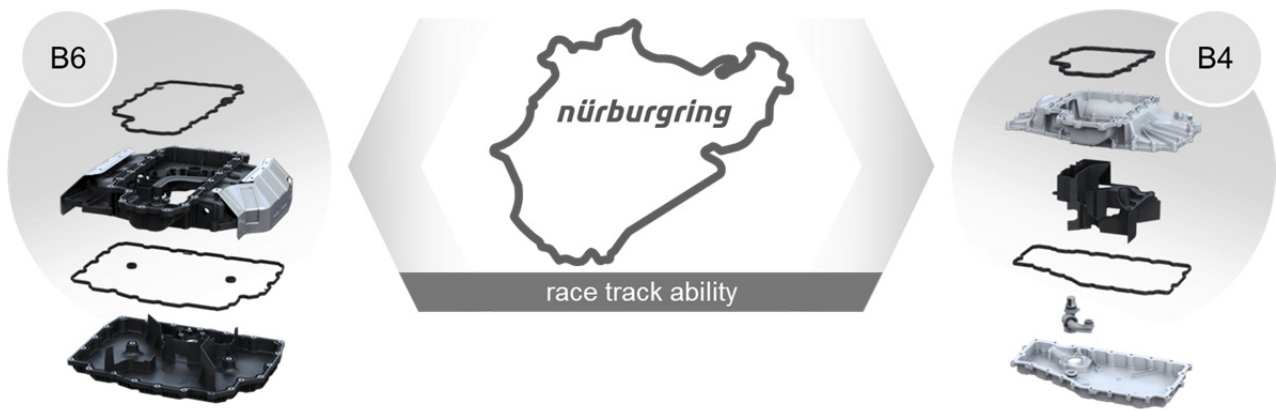
Figure 22: Flat-six and flat-four with integrated dry sump
